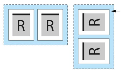
With an output from imposition process template, the concept is basically the same, except that instead of using the outside of the page placement layout, Prinergy Evo uses the device size defined in the imposition from Preps software. Rotating the imposition sheet swaps the dimensions of the generated file.
