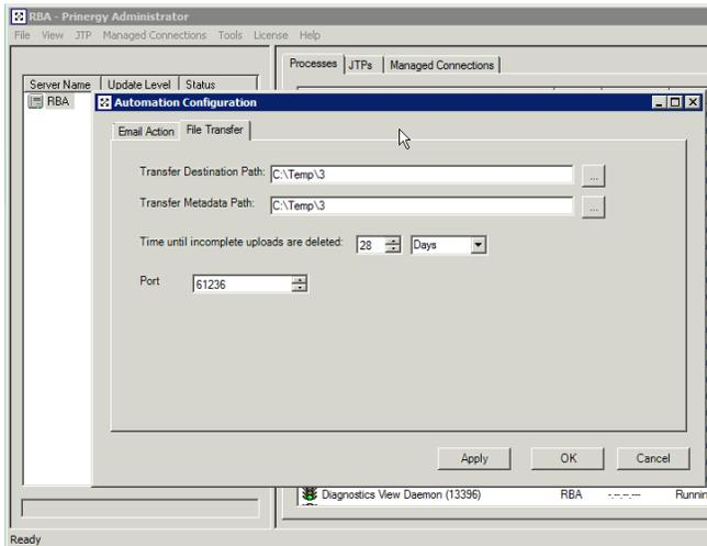
The system settings for the **Transfer Files** action are on this tab. There is no need to change anything in this dialog, as the defaults will work as supplied.
