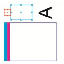
**Width Fit**: After choosing **Fit**, according to the location of the marks the software will adjust the width of the mark to be consistent with the length or width of the object which is going to be marked. The **Extra Length** option can be used to change the width of the mark. Users can set the value with formula.
