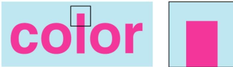
The text shown in the example is small—the letter l measures approximately 0.5 points across. With 100 percent trapping at a trap width of 0.3 points, the trap is so wide that the letter appears to be overprinting. When the trap is scaled to 25 percent, the trap is more appropriate to the size of the text.
