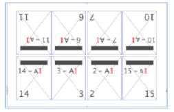
The paper is run through a press to print the front side of the sheet. It is then turned over on the vertical axis and run through the press again using the same gripper edge, and a second plate is used to print the back side of the sheet.
