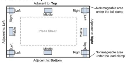
The following diagram shows sheet marks placed on a press sheet.
