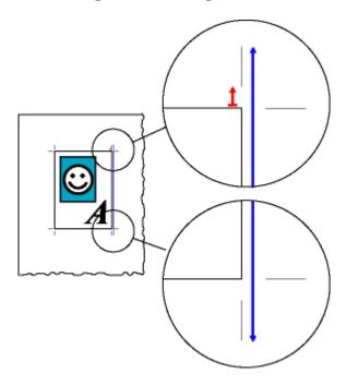
The long blue arrow indicates the **Locate crop mark of length** measurement. The short red arrow indicates the **at Distance** measurement.
