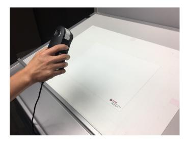
**Tip:** To reduce shadows when measuring the light booth luminance, make sure that the white reference paper is lying flat on the table top surface of the light booth. Then, position the colorimeter at a 45 degree angle to the reference white paper at a distance of 8-10 inches.
